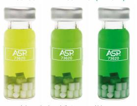
A slower color change indicates an area with less cavitation energy or a "weak point" in the cleaning tank, while a failure result indicates a "cold spot" or an area without sufficient cavitation energy.
