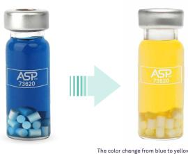
The color change from blue to yellow indicates the presence of cavitation energy. The time taken for this color change indicates the level of energy and degree of cavitation provided by the ultrasonic cleaner in that location.
