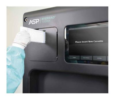
Cassettes are sealed, so the user is not exposed to any risk. The container incorporates a chemical indicator designed to detect all leaks of the sterilizing agent.
